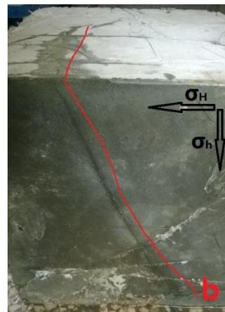
*Fig.4 Fracture propagation when perforation orientation is 60°*
