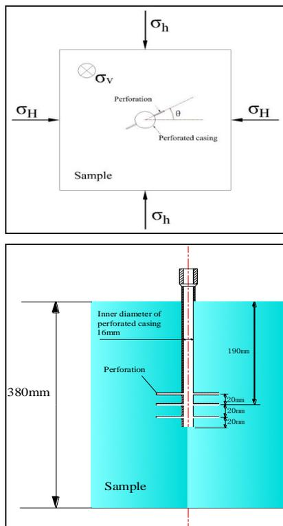
Fig.2 Plane sketch of synthetic sample
