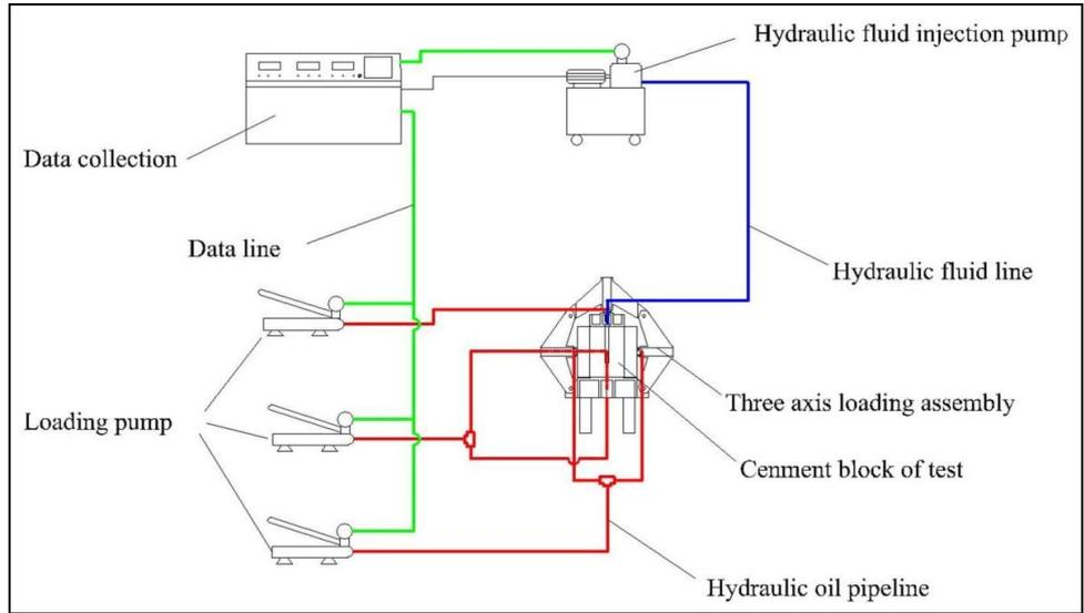
Fig.1 Sketch map of three axis hydraulic fracturing simulation system
