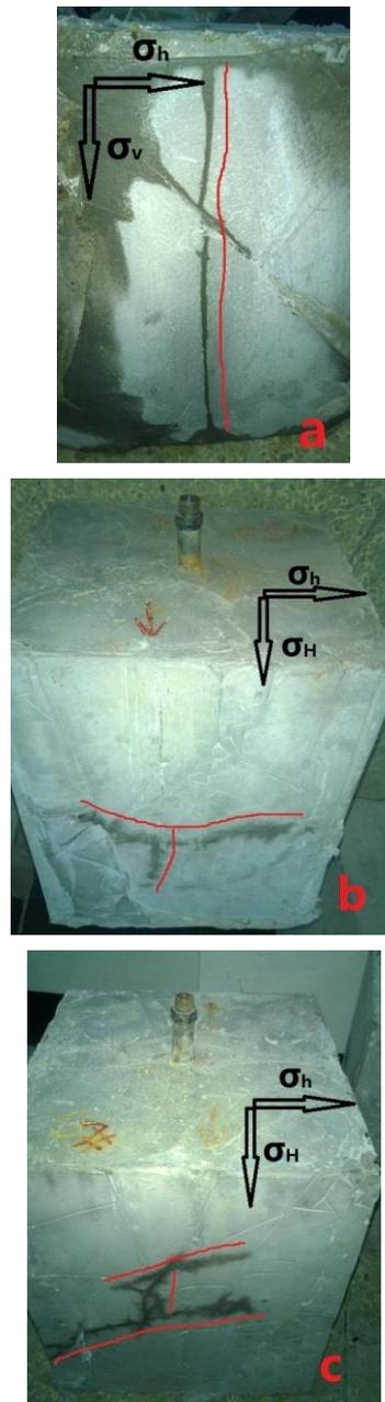
**Fig.3** Fracture propagation when perforation diameter is 6mm, 8mm and 10mm
