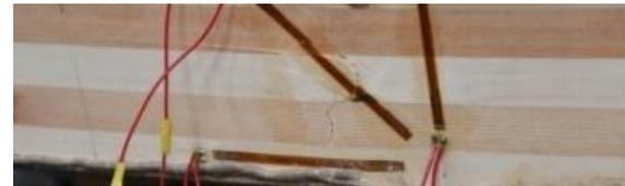
Figure 9.The strain gage was broken in tension stress
