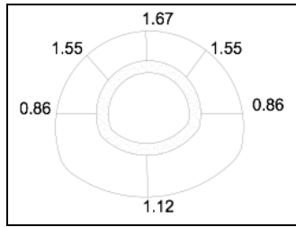
Figure 16. Water pressure of 8m thickness (MPa)
