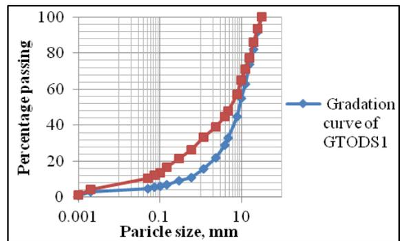
Figure 12. Change in gradation of OB dump material GTODS1 with the addition of fly ash
