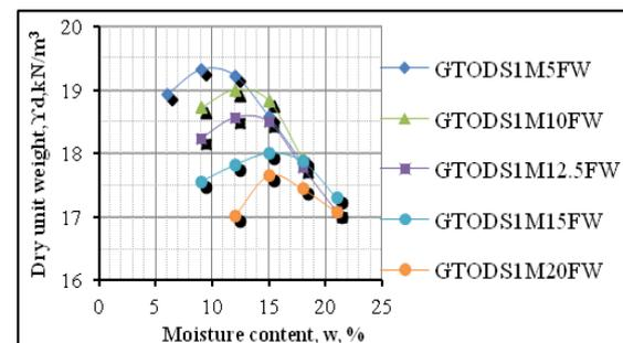
*Figure 3. Effect of increasing fly ash content on compaction behaviour of GTODS1*
