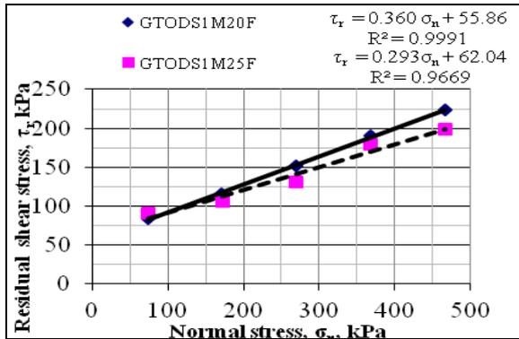
Figure 11. Residual shear strength envelope of GTODS1 mixed with 20% and 25 % fly ash by volume
