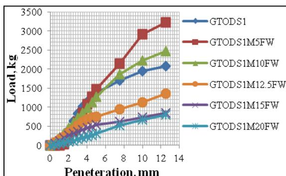
**Figure 4.** Load vs penetration curve of unsoaked condition
