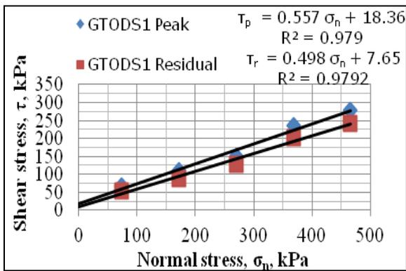
Figure 6. Mohr-Coulomb failure envelopes for dump material sample GTODS1 at OMC
