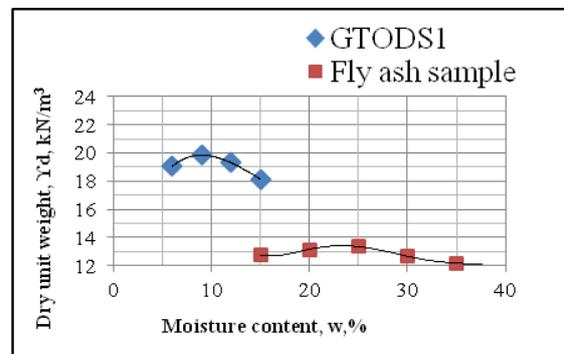
*Figure 2. Compaction curves of fly ash and OB dump material sample GTODS1*
