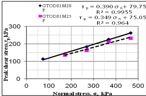
Figure 10. Peak shear strength envelope of GTODS1 mixed with 20% and 25 % fly ash by volume
