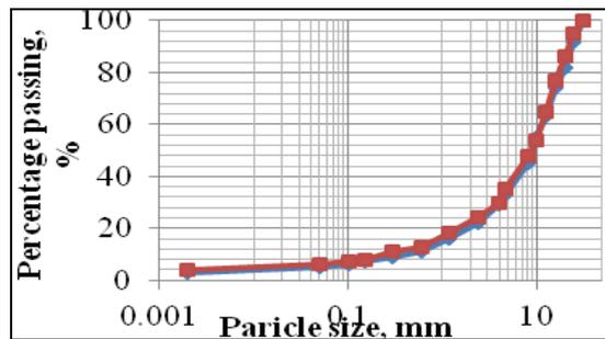
Figure 9. Gradation curves of dump material sample GTODS1 before and after the shear test conducted at normal stress of 172 kPa
