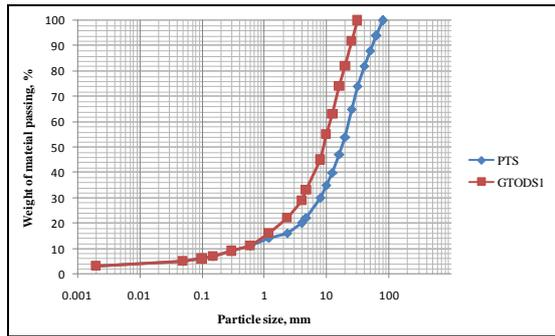
**Figure 1.** Gradation of the prototype sample and prepared OB dump material sample GTODS1
