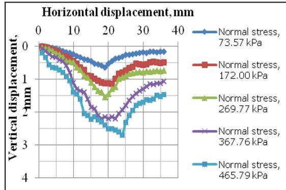
Figure 8. Horizontal displacement versus vertical displacement curves for OB dump material sample GTODS1 at OMC
