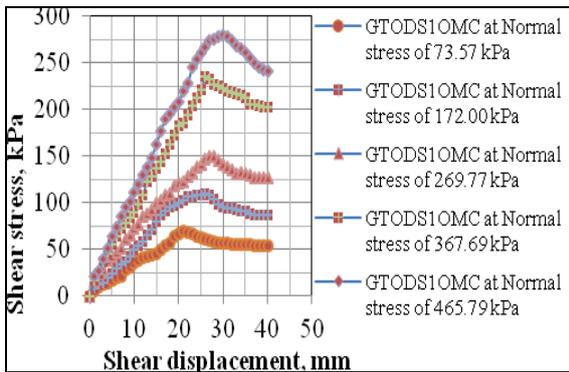
Figure 7. Shear stress versus horizontal displacement curves for dump material sample GTODS1 at OMC
