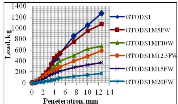
**Figure 5.** Load vs penetration curve in soaked condition
