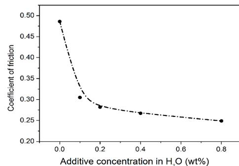
**Figure 6.** Coefficient of friction for various concentrations of carbon beads in water under 1.0 N normal load (Sliding speed : 5 cm/s, rotating diameter: 1 cm)
