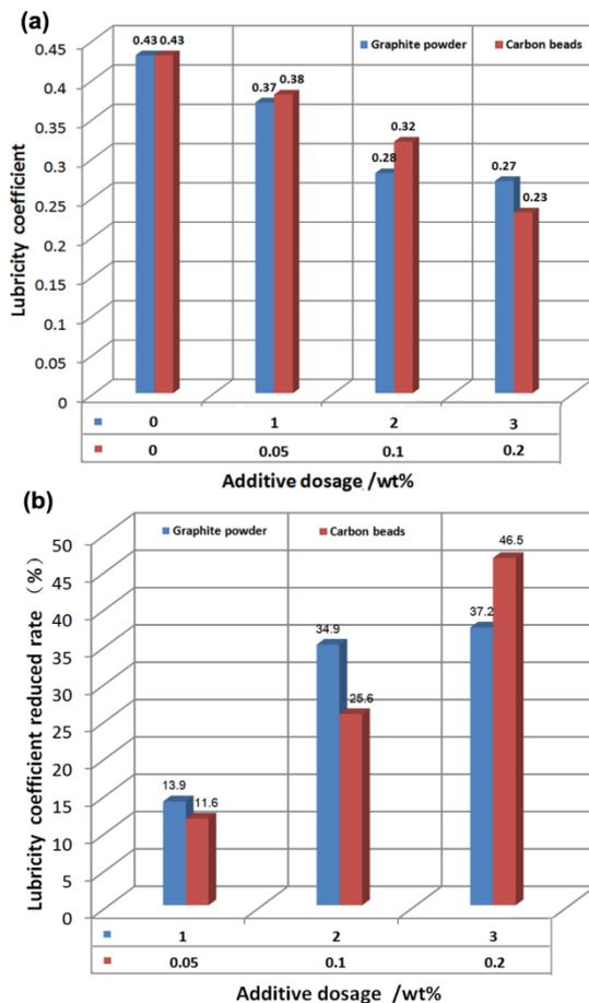
**Figure 4.** Lubricity coefficient (a) and lubricity coefficient reduced rate (b) of graphite powder and carbon beads in bentonite suspension (1 wt %) with different concentrations
