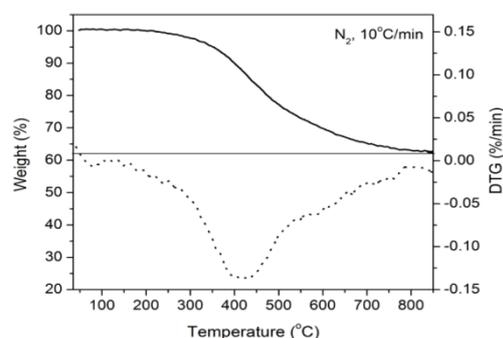
**Figure 3.** TG and DTG curves of colloidal carbon beads in nitrogen atmosphere
