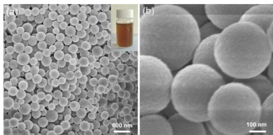
**Figure 1.** SEM images of colloidal carbon beads. Insert is carbon beads aqueous solution
