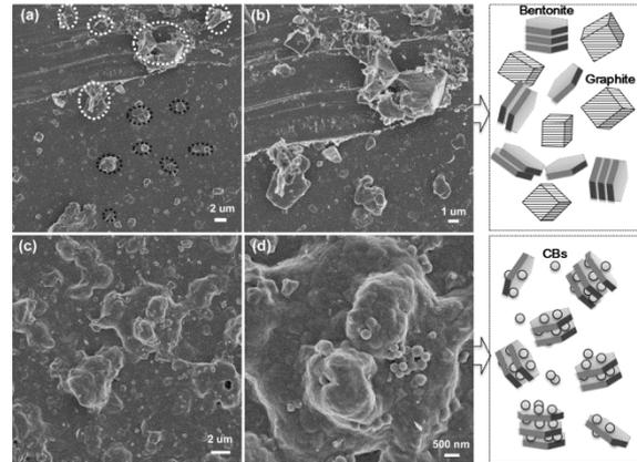
**Figure 5.** SEM images of bentonite/graphite and bentonite/CBs suspension dropped on silicon wafer and dried at room temperature
