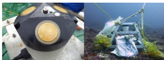
Figure 6. ADCP and the stabilizing steel frame
