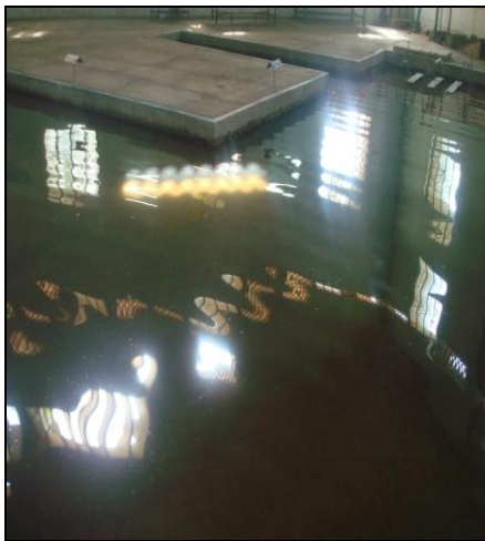
Figure 7. Model Photo showing wave crest near Proposed Flotilla Berths
