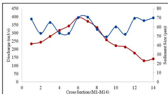
Figure 8. Average sediment size variation with discharge
