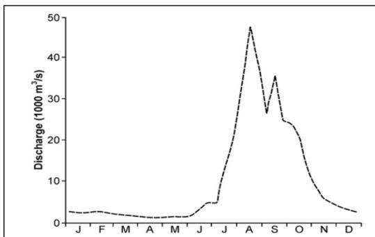
Figure 4. Hydrograph of river Ganga (Source: Singh et al., [33])
