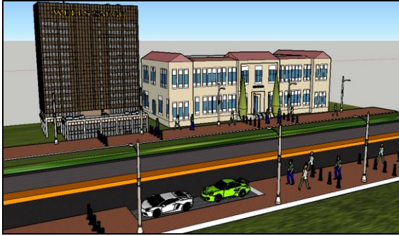
Figure 17: Table Top Crossing and Cycle Track (in orange colour) at the Intersection at the starting of Reach 2
