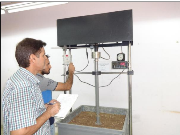
Fig.9: Carrying out cyclic load test
