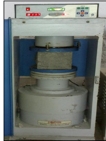
Figure 2: Compressive strength of cubes
