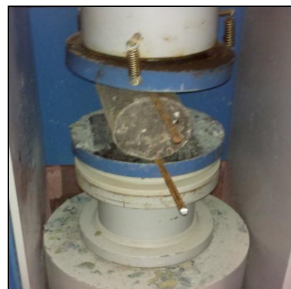
Figure 4: Split tensile strength of cylinders
