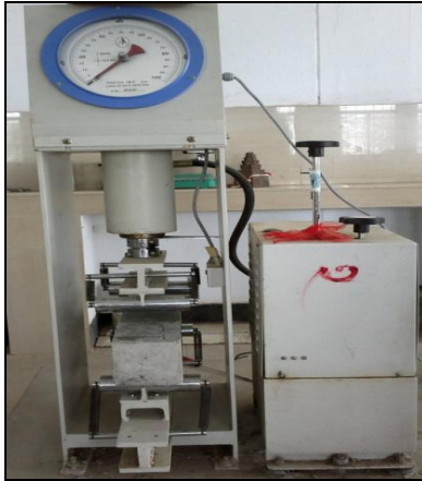
Figure 5: Flexural strength of prisms
