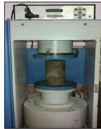
Figure 3: Compressive strength of cylinders
