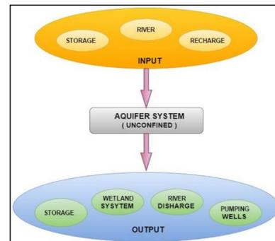
Figure 8. Schematic representation of water budget of the aquifer in the study area
