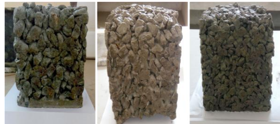
Figure 5: Samples of no-fines concrete cube having varying size of aggregates (w/c ratio= 0.45; cement-aggregate ratio=1:5)
