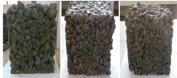
Figure 4: Samples of no-fines concrete cube having varying size of aggregates (w/c ratio= 0.40; cement-aggregate ratio=1:5)
