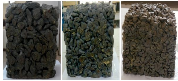
Figure 3: Samples of no-fines concrete cube having varying size of aggregates (w/c ratio= 0.35; cement-aggregate ratio=1:5)
