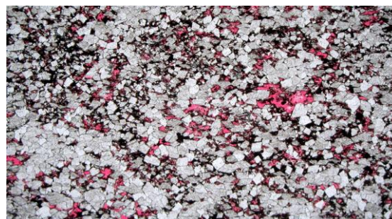
Fig.5 Intercrystalline dissolution pores (Maoba4 well, T1f1)
