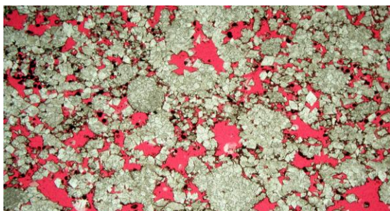
Fig.4 Oolitic dissolution pores (Maoba4 well, T1f2)
