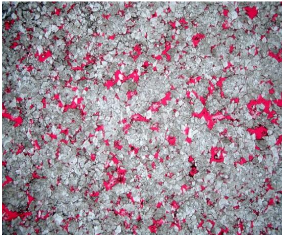
Fig.2 Residual Oolitic dolomite (Dawan 102 well, T1f2)
