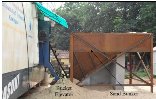
Fig. 5: Photograph of sand bunker feeding sand to bucket elevator
