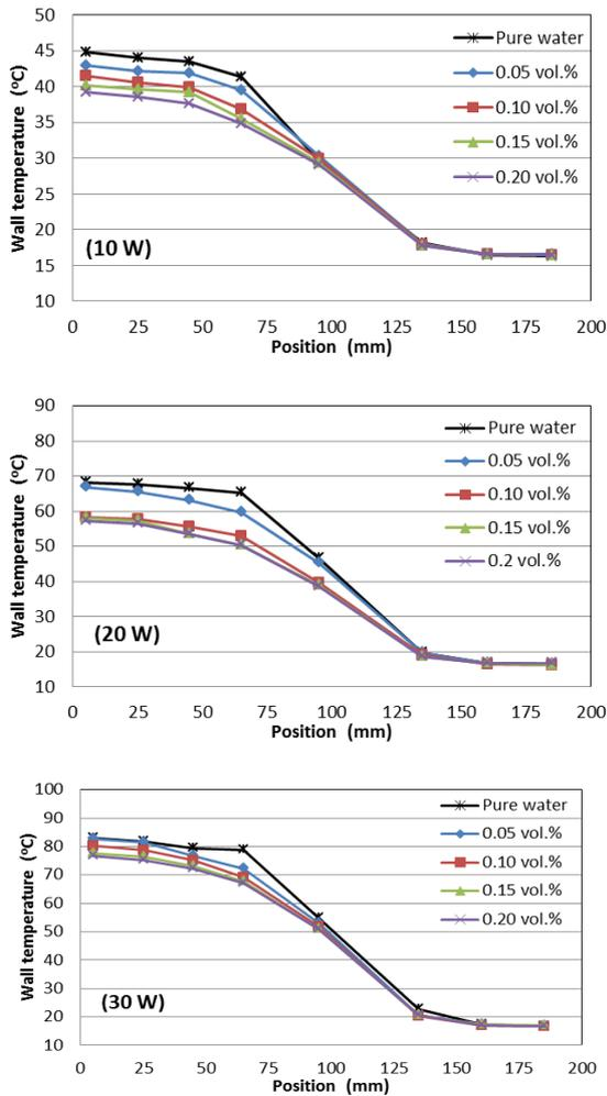
Fig. 2 Effect of GO concentration on the wall temperature distribution at input power levels of 10, 20 and 30 W
