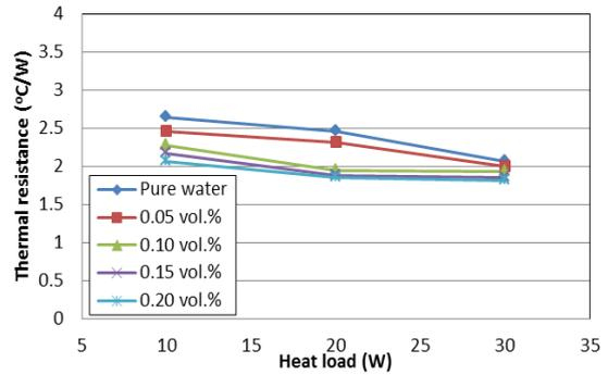
Fig. 3 Thermal resistance as a function of concentration and input power
