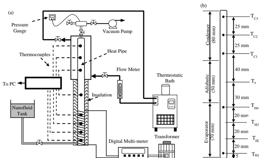
Fig. 1 (a) Schematic diagram of the experimental apparatus, (b) locations of the thermocouples
