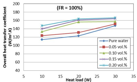
Fig. 4 Overall heat transfer coefficient as a function of concentration and input power
