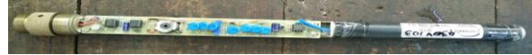
Figure 1: Logging probe hosting Geiger Muller counter and associated electronics used for gamma ray spectra in a borehole
