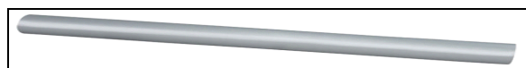
Figure 5d: Non Collapse of stainless steel tube of 0.6 mm thickness that buckles at 55 kg/sq.cm.
