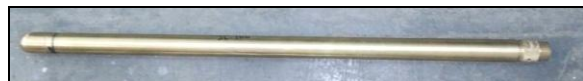
Figure 5c: Non Collapse of brass tube of 1.6 mm thickness that buckles at ~ 98 kg/sq.cm.
