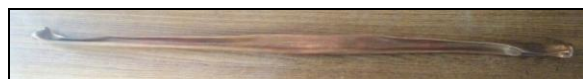
Figure 5a: Collapse of copper tube of 0.6 mm thickness buckled at 20 kg/sq.cm. Brass
