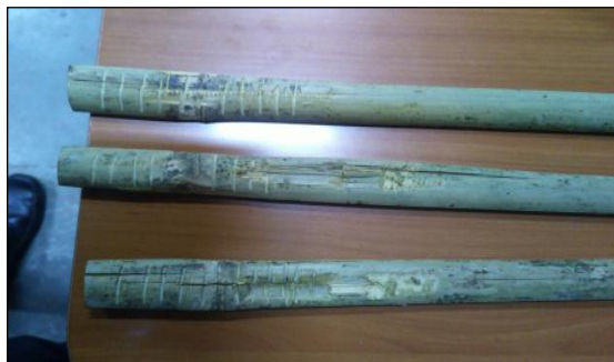
Figure 7. Failure of splints in tension
