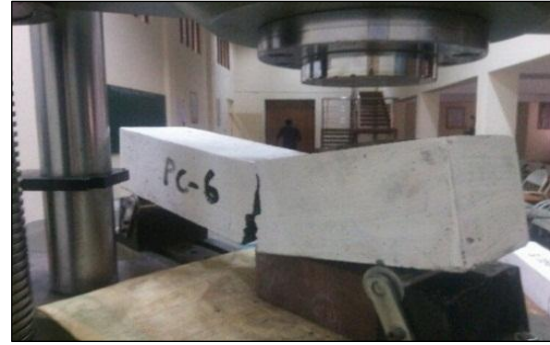
Figure 12. Crack formation in RC beam
