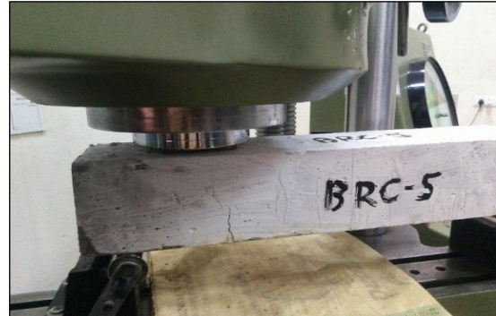
Figure 13. Cracks in BRC beam
