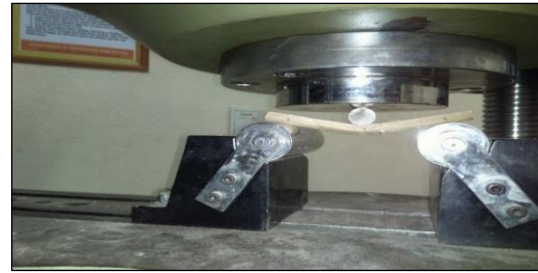
Figure 8. Static bending test on bamboo splint
