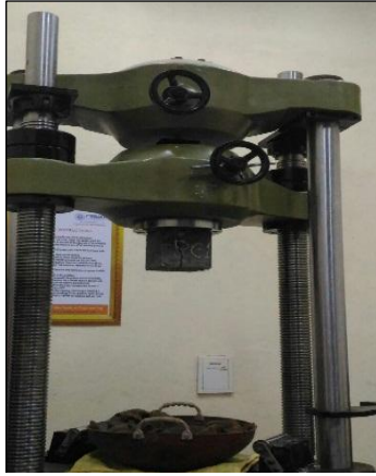
Figure 6. Pull out test setup
