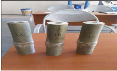
Figure 2. Bamboo culms with node for compressive test
