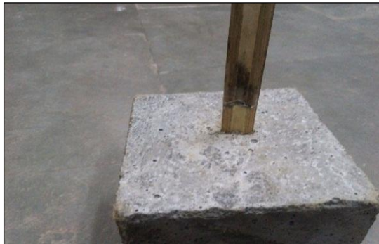
Figure 15. Slip in BRC cube
