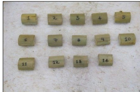
Figure 1. Bamboo specimen for density test
