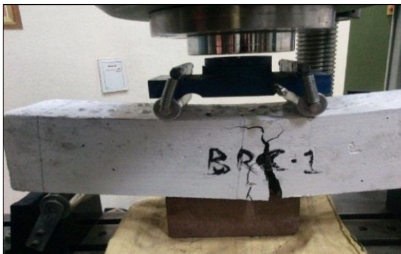
Figure 10. Failure of BRC beam in flexure
