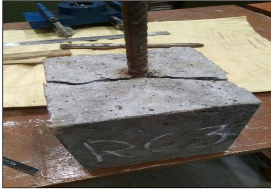
Figure 14. Failure of RC cube
