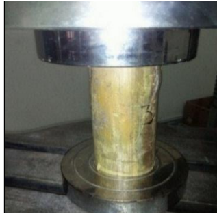
Figure 5. Poisson's ratio test
