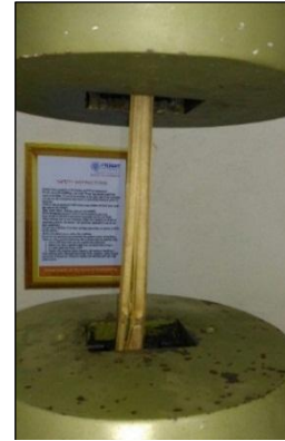
Figure 4. Tensile testing of bamboo
