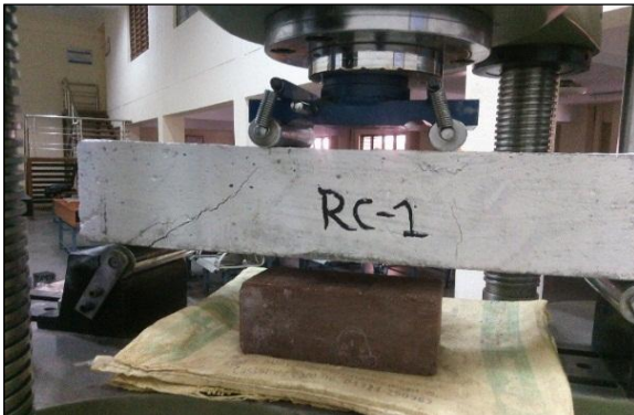
Figure 11. Crack formation in RC beam
