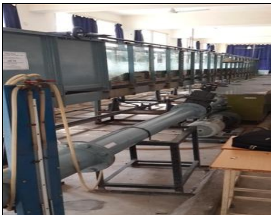
Figure 1: Experimental Setup: Tilting Flume
