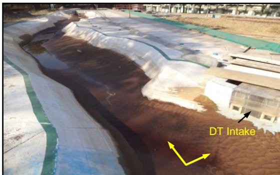
Figure 7: Deposition when DT is in operation
