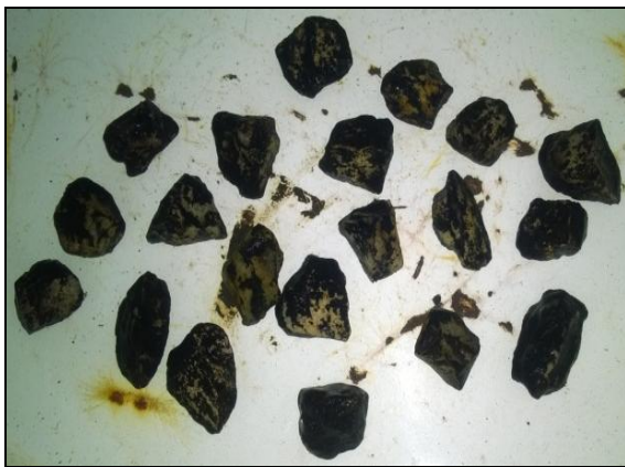
Figure 5: Stripping of Type 2 Aggregate under Alkaline Condition pH 11 with Pressure
