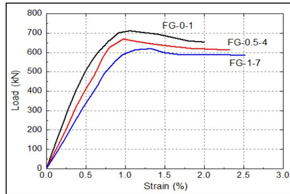
Figure 5: Load-axial compression strain of stub columns
