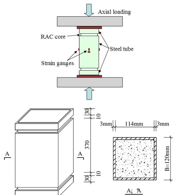
**Figure 2: Layout of test setup and cross-section of RACFSST columns**
