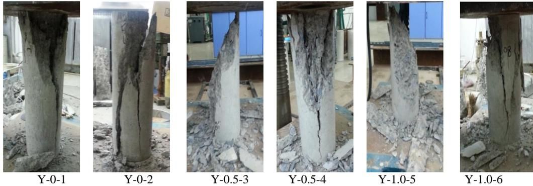
**Figure 1: Failure modes of RAC columns**
