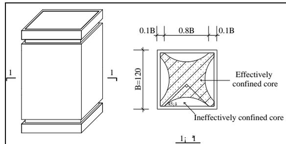
Figure 6: Effectively Confined Core for RACFSST columns
