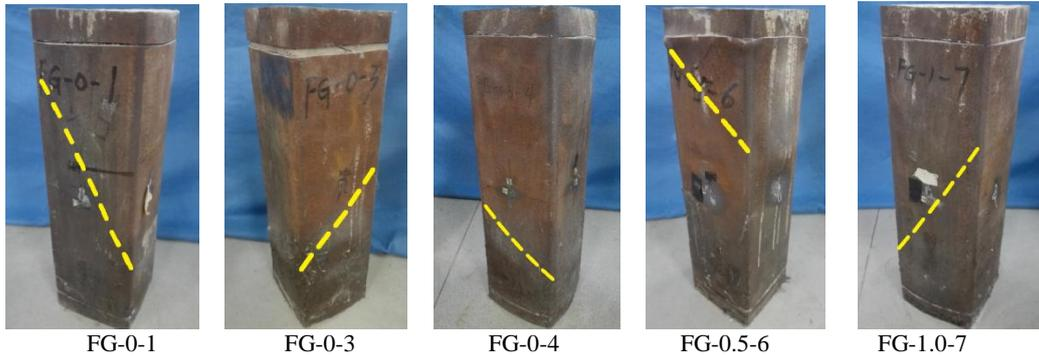
Figure 3: Failure modes of representative RACFSST specimens
