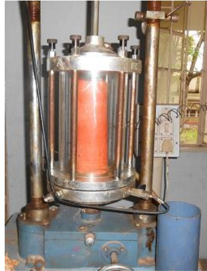
Figure 3 Tri-axial Test Setup
