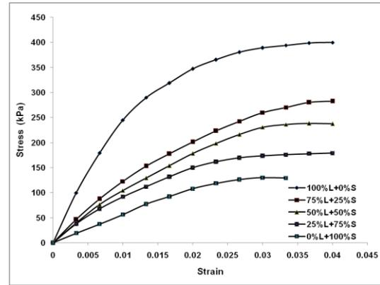
Figure 12 Stress-Strain Graphs for UCS at Optimum Moisture Content
