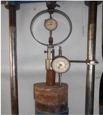
Figure 2 UCS test setup
