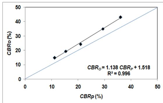
Figure 9 Plot of Observed CBR Vs CBR Predicted based on the angle of internal friction
