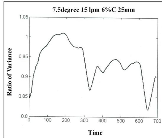
**Figure 6:** Variance-ratio curve for detection of unhealthy region of pressure signature at fixed window size
