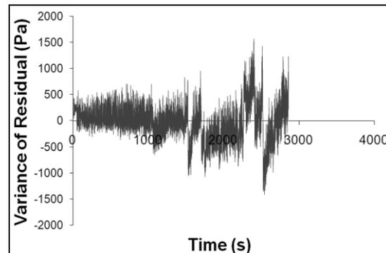
**Figure 7:** Curve of time against residual pressure obtained after trend removal
