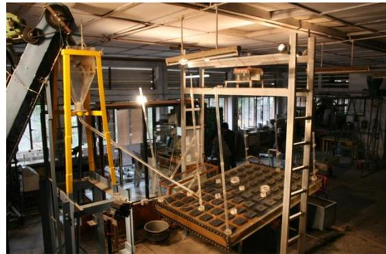
*Figure 1: Photograph of the experimental set-up used for gravity blind backfilling*
