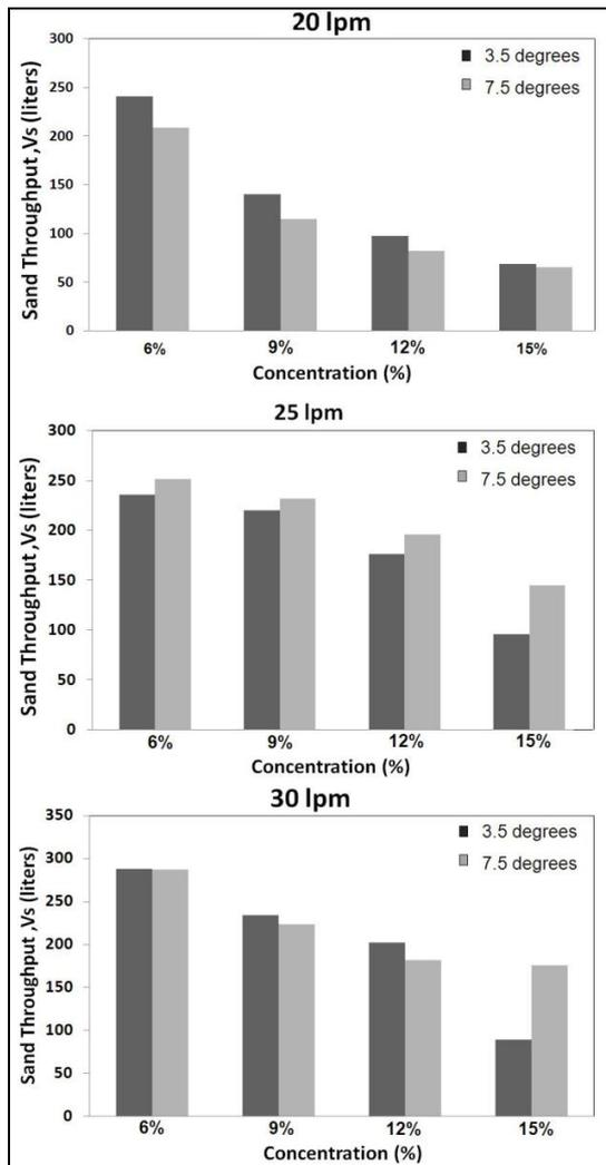
Figure 3: Comparison of sand throughput at 7.5° and 3.5° model inclinations
