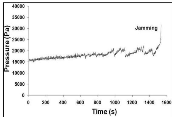
Figure 4: Pressure-time curve recorded by the data acquisition system during the filling process
