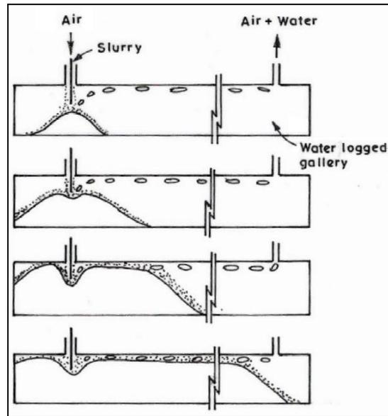
Figure 2: Sequence of the filling process
