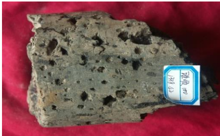
Figure 3: Solution pores in basalts of Kongdian Formations in Shengshun 100 exploratory well
