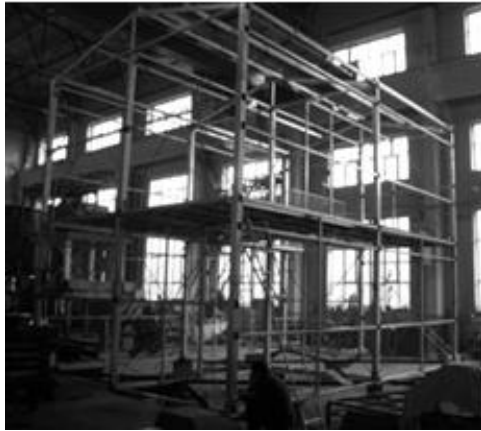
Figure 1: Photo of shaking table test specimen
