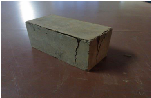
Fig. 5 Failure planes after compression
