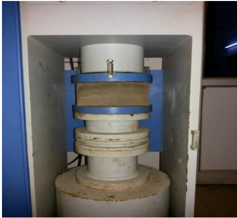
Fig. 4 Testing of bricks for its compressive strength
