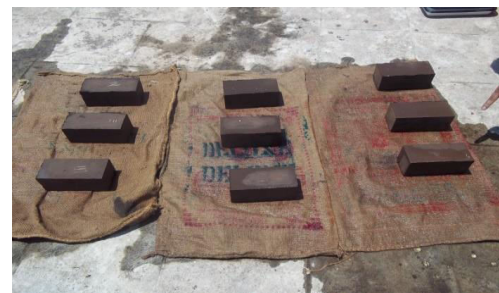
Fig. 3 Curing of bricks
