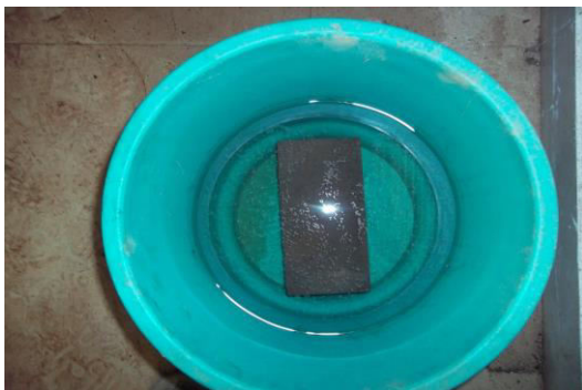
Fig. 6 Water absorption test on prepared bricks
