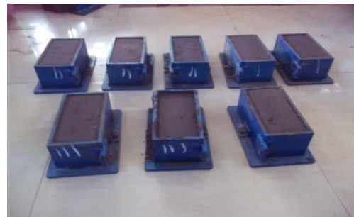
Fig. 2 Mixture filled in bricks mould
