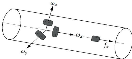
Figure 2. Inertial navigation system consisting of gyroscope and accelerometer
