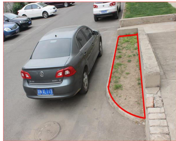
Figure 2: Experiments for gully erosion measurement: the area within the red line was simulated as the gully area in the experiment, and the black car was used as a reference.
