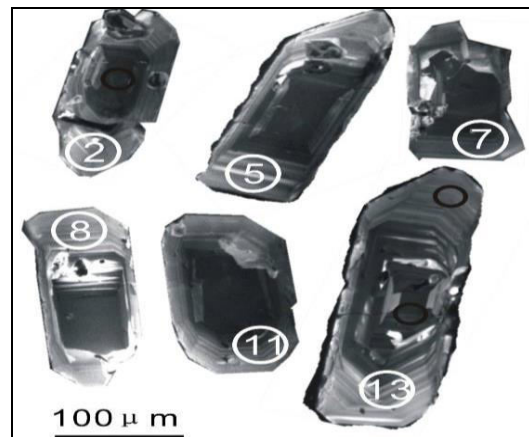
Fig. 4 Representative CL images of zircon of granite in the Bianjiadayuan Pb-Zn-Ag deposit for in situ Hf isotope analysis
