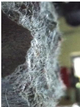
Plate 7: Distribution of Glass Fibers in failed fiber reinforced GPC Prism
