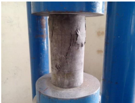
Plate 6: Failure of fiber reinforced GPC Cylinder with 0.03% fibers in compression
