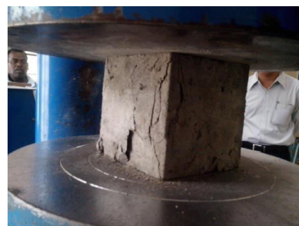
Plate 5:Failed Glass Fibered GPC Cube
