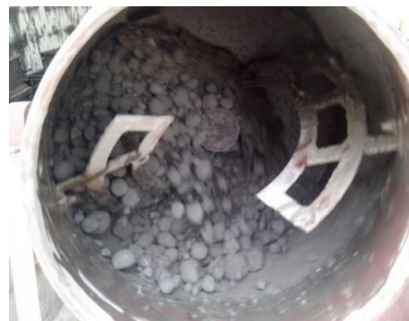
Plate 4 : Balling Effect at 0.03% of fibers by volume of concrete
