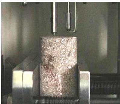
Fig 2: ATA-IGG I type rock abrasion servo tester
