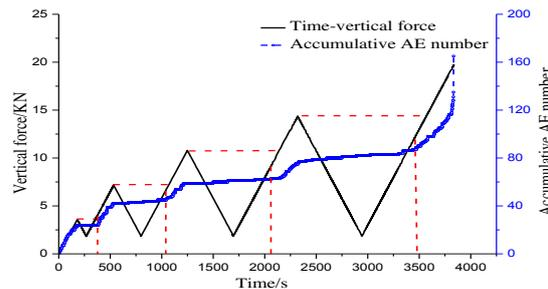
**Figure 5. Time-vertical force-accumulative AE number curve**
