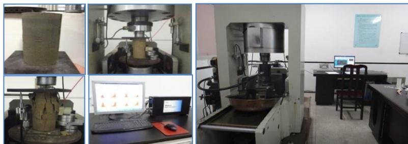
*Figure2. Sample of filling body and test system*
