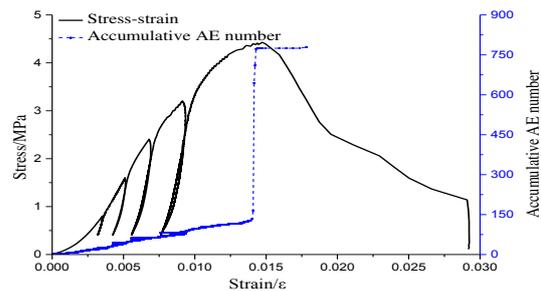
**Figure4. Stress-strain-accumulative AE number curve**
