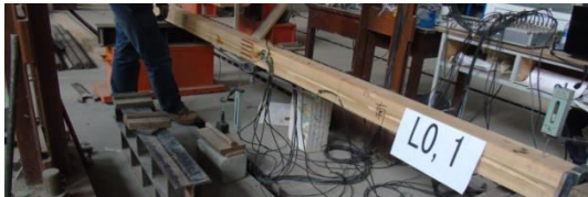
Fig.8 The picture of beam before load test
