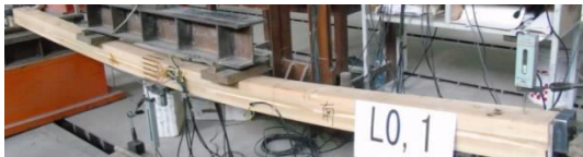
Fig.9 The picture of beam after load test
