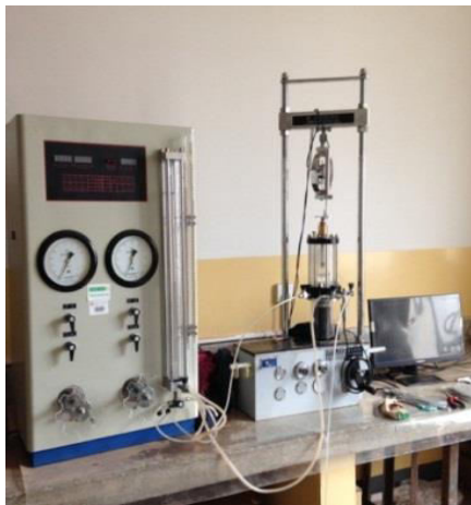
Fig 5: TSZ30-2.0 triaxial strength test instrument with strain control
