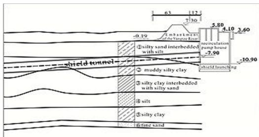
**Figure 1.** Sectional view of strata crossed by shield tunneling
