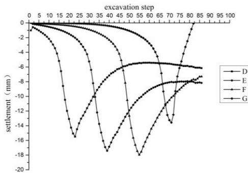
Figure 6. Settlement of tunnel
