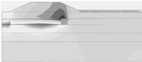
Figure 3. Vertical displacement nephogram
