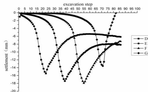
Figure 5. Ground settlement of embankment
