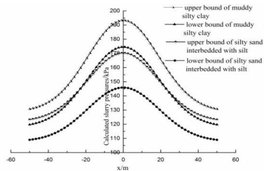
Figure 7. Calculated slurry pressures
