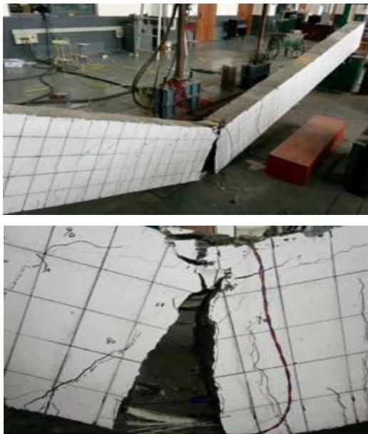
Figure 4. The failure mode of beam
