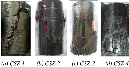
Fig.6. Coal specimen failure photos of conventional triaxial experiment
