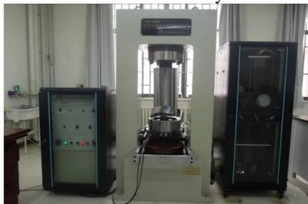
*Fig.1. TAW-2000 rock mechanics experimenting machine*
