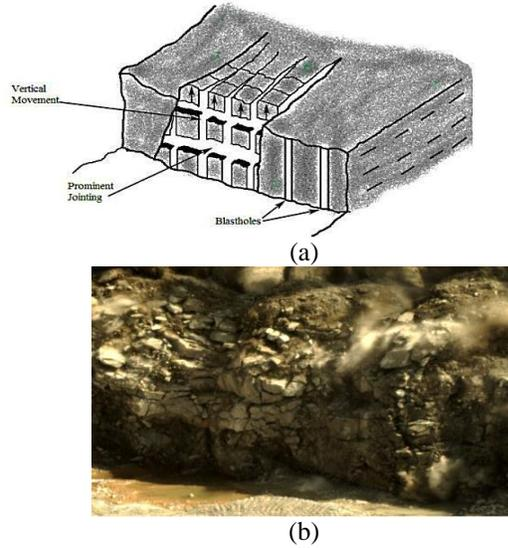
**Figure 14.** Rock fragmentation affected by jointing (recorded by HSC)
