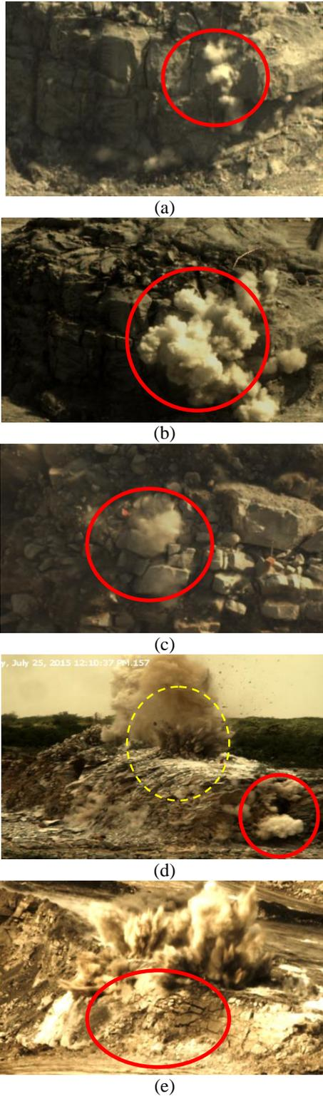
**Figure 13.** Escape of gas energy through weakplanes & stemming zone
