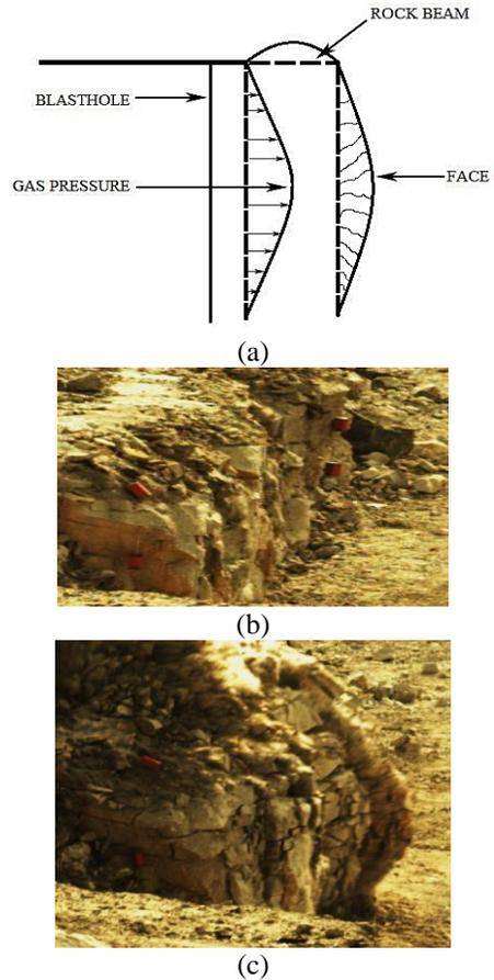
**Figure 15.** Flexural bending mechanism
