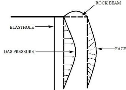
Figure 3. Rock breaking by flexural bending (Ash, 1973)
