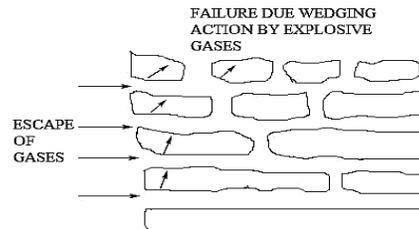
Figure 4. Escape of gases into joints
