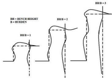
Figure 12. Bending conditions in blasting (Smith, 1976)
