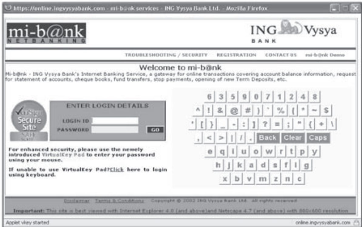
Fig. 13 – An example of dynamic electronic keyboard
