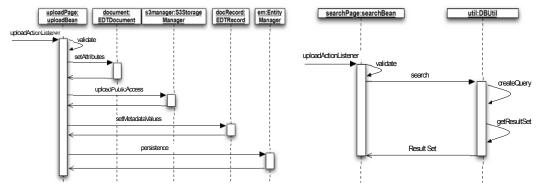
Figure 8. Upload process sequence diagram.
