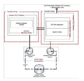
Figure 4. Single instance cloud deployment.
