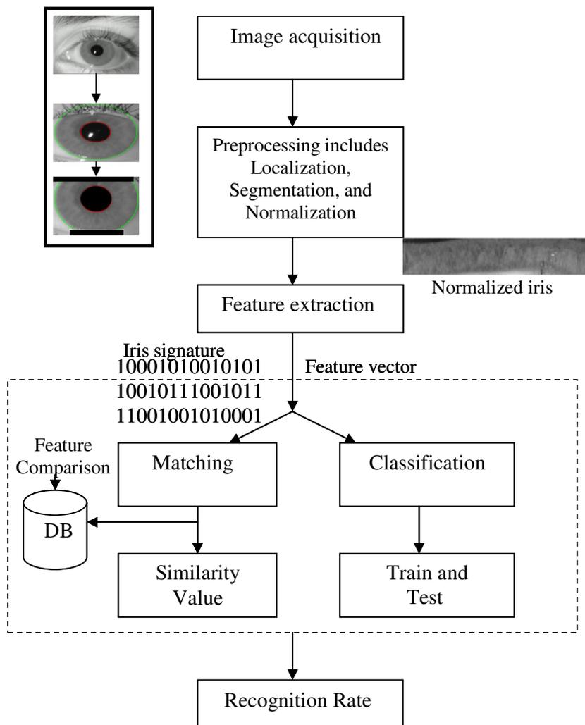
Fig. 1. General structure of Iris Recognition System.
