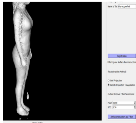
Figure 4.1: Result using Greedy Triangulation
