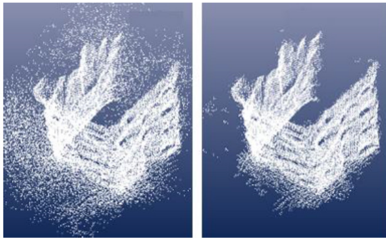
Figure 3.4.3: Demonstration of Statistical Outlier Removal Filter
