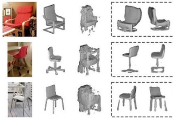
Figure 13. 3D construction of chairs on IKEA dataset. From left to right: input, ground truth, 3D estimation by 3DGAN and two view of MarrNet [48]
