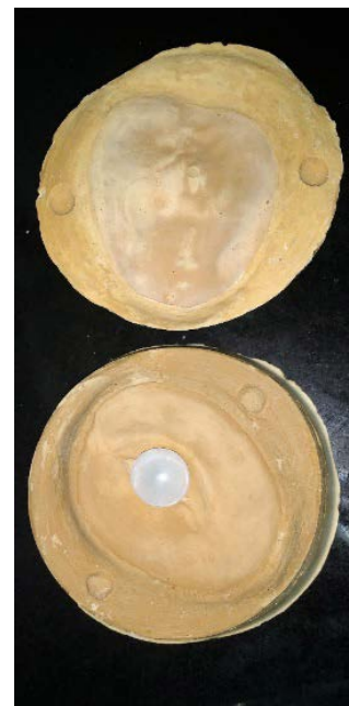
Figure 5: Two part mould with fixed eye shell after dewax
