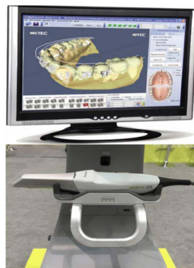
Figure 1. Parts of intraoral scanner - Computer monitor, hand held camera wand.
