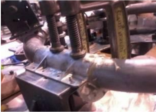
a) Master brackets clamped on jig with resin
