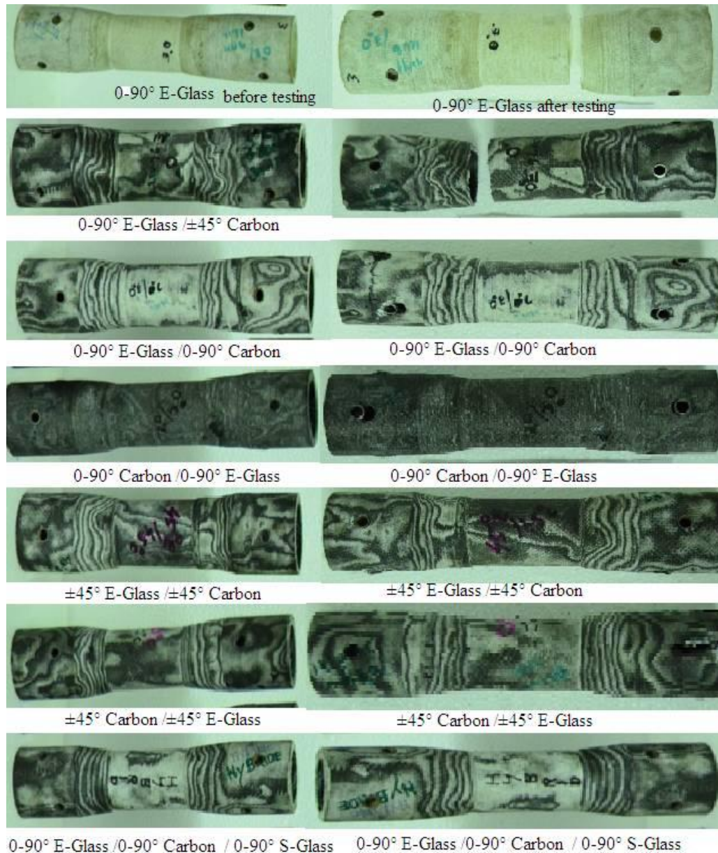
Fig. 1: Composite drive shaft specimens before & after tensile test
