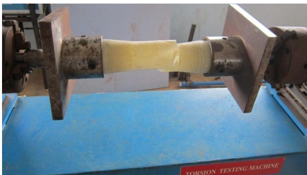
Fig. 4(a): Torsion test setup and composite drive shaft specimen
