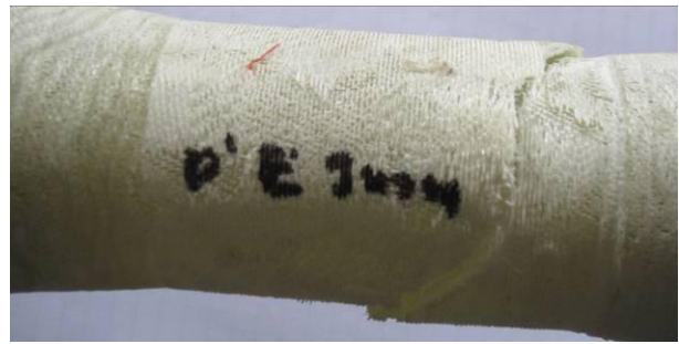
Fig. 4(b): Composite drive shaft specimen failed in torsion test
