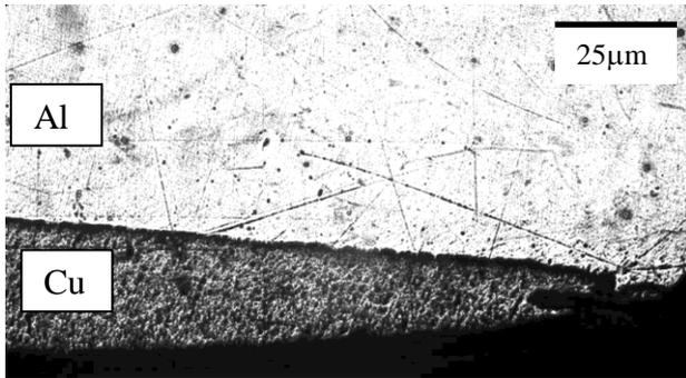
Fig. 4(a): Microstructure of Al/Cu MPW weld sample
