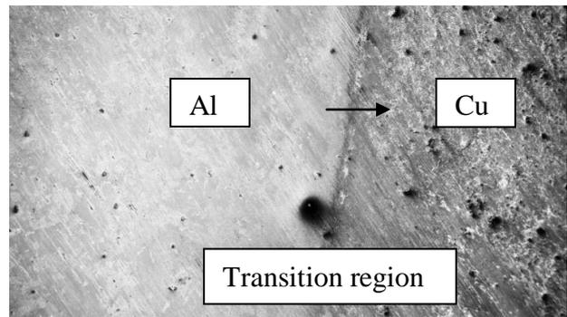
Fig. 5: SEM image of Al/Cu welded specimen
