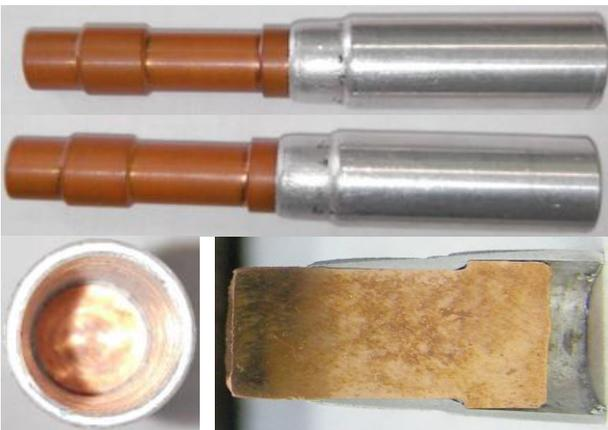
Fig. 2: MPW Specimen and their views of cross section & weld top
