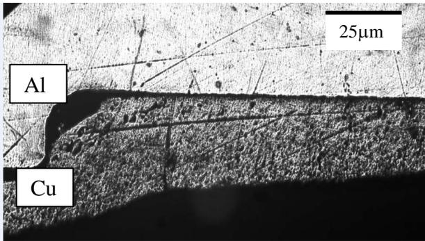
Fig. 4(b): Microstructure of Al/Cu MPW weld sample
