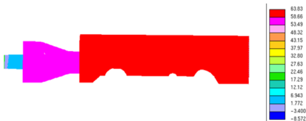
Fig. 9: STB design - Pressure (in Pa) distribution
