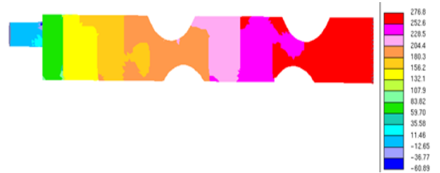
Fig. 11: LT design - Pressure (in Pa) distribution
